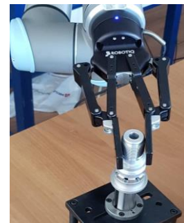
Figure 4. UR10 manipulator robot with 2F-140 adaptive gripper
