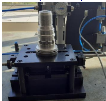
Figure 3. Inner diameter measurement system
